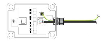
5. Connect the network cables to RJ45 connectors.
